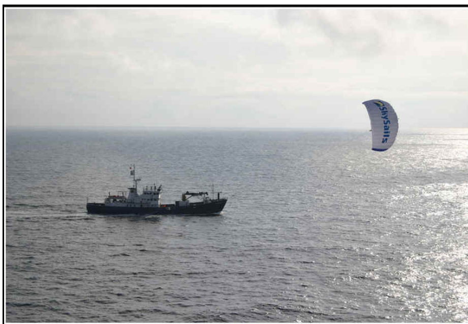
Figure 3: A cheaper way to transport freshwater over the ocean. The world's first commercial merchant ship pulled by a giant high-tech kite aiding its engines to slash fuel consumption and cut greenhouse gas emissions was launched in Hamburg, 14 th December 2007. The SkySails system purports to be able to lower a ship's annual average fuel costs by between 10% and 35%. 49
